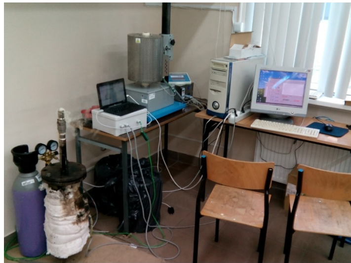
Fig.2.14.a A Experimental stand for the slow pyrolysis process
