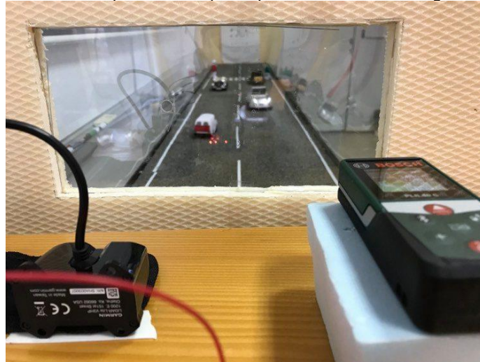
Fig. 7. Evaluation of lidar and rangefinder results in different fog conditions
