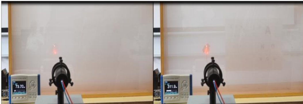
Fig. 5. Fog layer configuration: a) Dense fog conditions; b) Conditions with moderate fog
