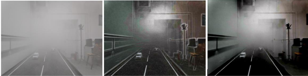
Fig. 9 Image with dense fog: a) original; b) fog removed; c) refined by applying DCP
