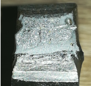
Fig. 4/5.6 Aspect of the sample welded with ER70
