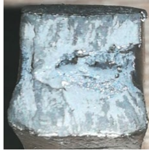
Fig. 7/5.9 6 Aspect of the sample welded with ER308
