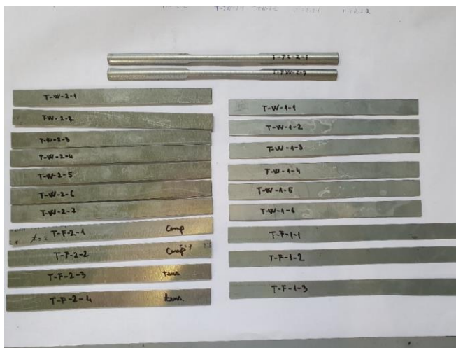
Fig. 13 Coupon test samples for material tests.
