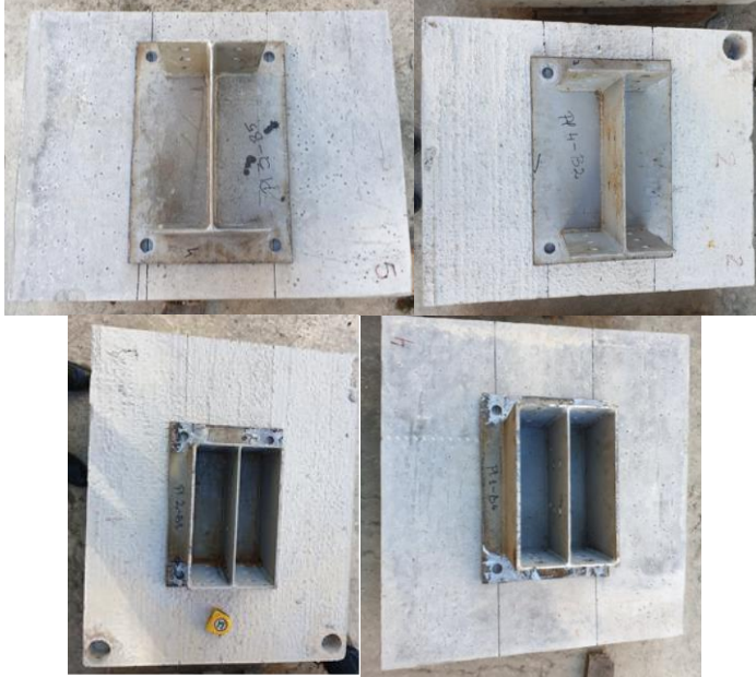
Fig. 12. Concrete-base assemblies used in experimental tests.
