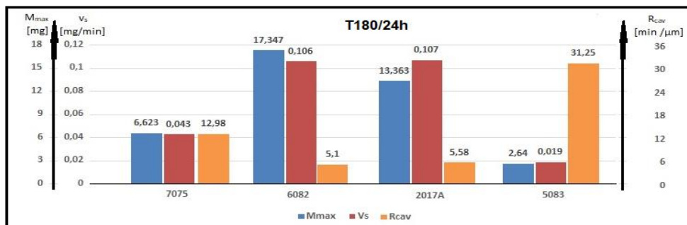
Fig. 7.4 Histogram of the comparison of parameters of resistance to cavitation erosion (180/24h treatments)
