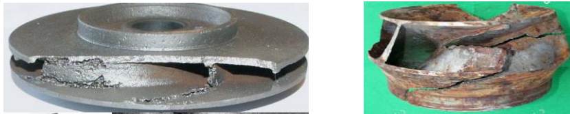
household pump impellers: a) cast aluminum alloy impeller [172], b) cavitation destroyed impeller [179]
