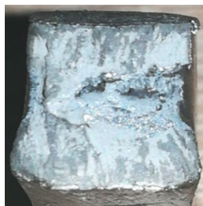
Fig. 7/5.9 Aspect rupere epruveta sudata cu ER308
