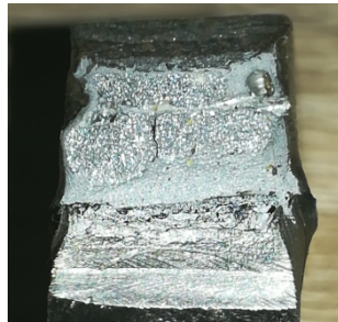
Fig. 4/5.6 Aspect rupere epruveta sudata cu ER70
