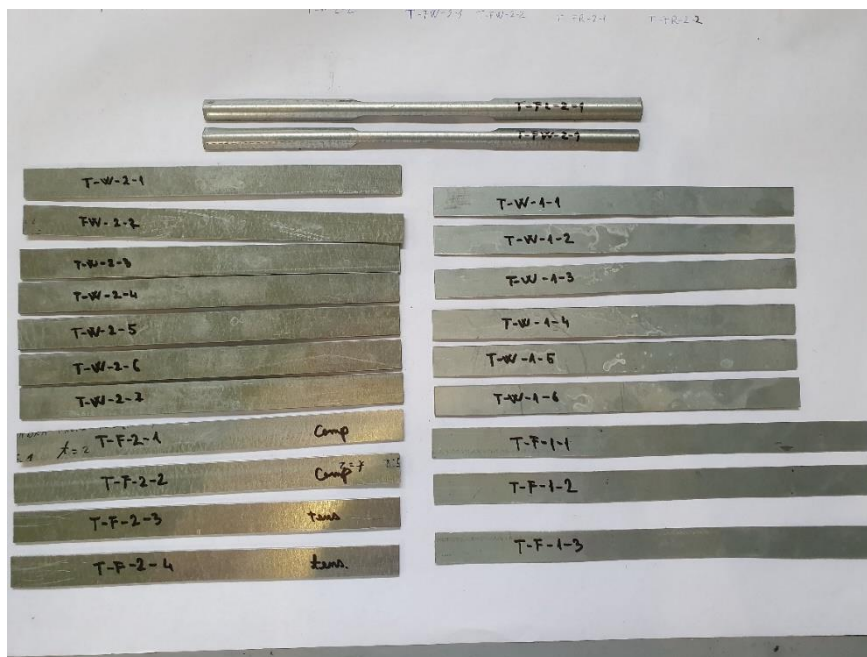
Fig. 13 Coupon test samples for material tests.
