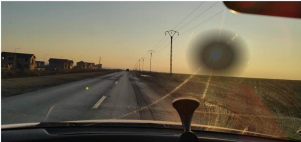
Fig. 3 Application of the sun visor in a case where the driver is affected by sunlight.
