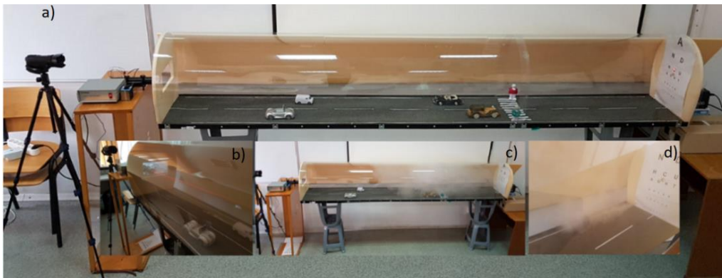
Fig. 12 Experimental system used to estimate visibility in fog.
