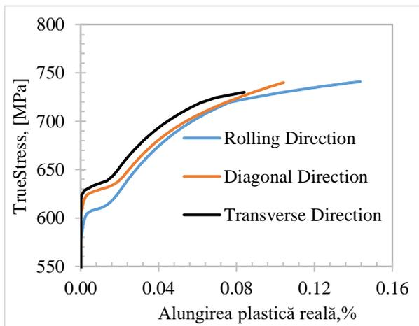
Fig. 9 Conventional Characteristic Curves and the Plasticity Region
