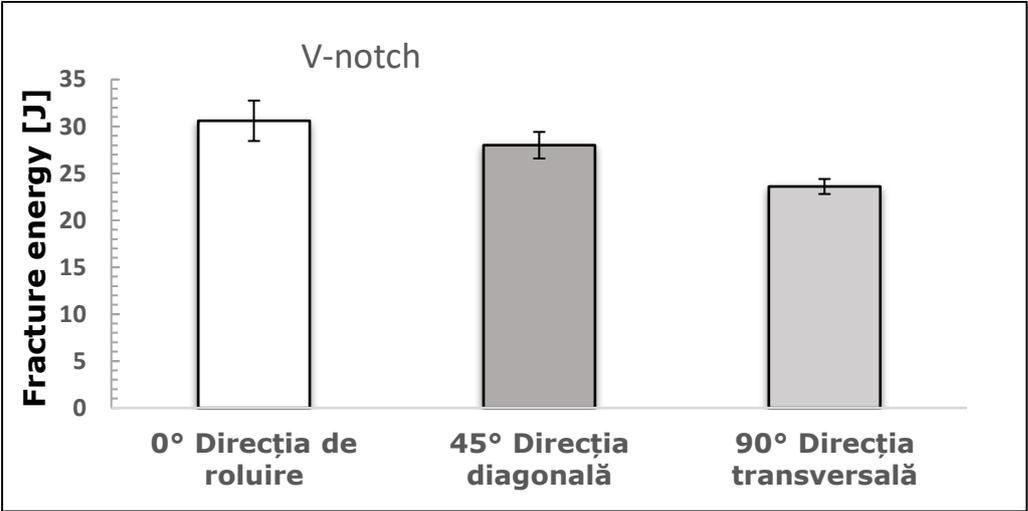
Fig. 11 Results of the Resilience Tests for V-Notched Specimens
