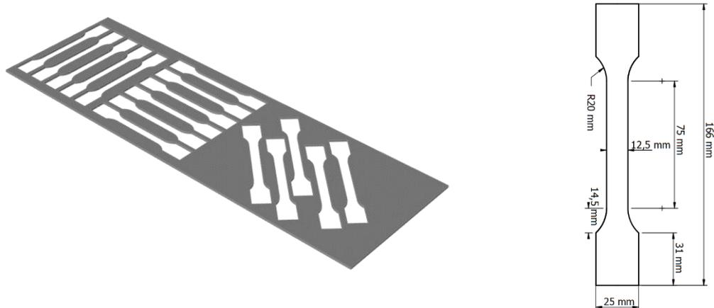
Fig. 7 CAD Sketch of the Test Specimen Orientations and Specimen Dimensions According to ISO 10113:2006 Standard
