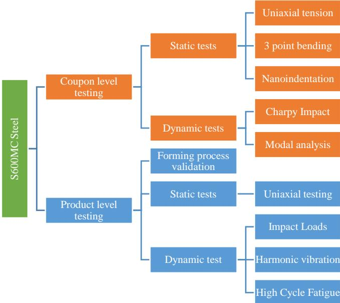
Fig. 3 Schematic Outline of the testing research program
