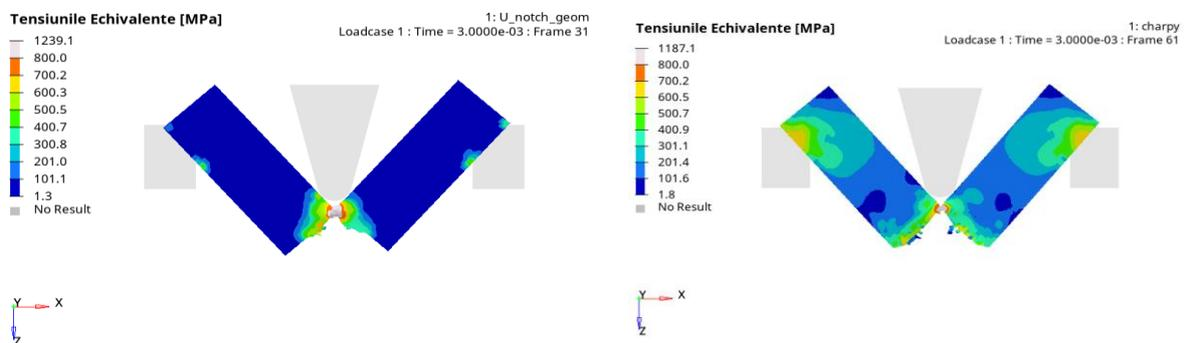
Fig. 14 Comparison of Equivalent Stresses During Resilience Tests for U-Notched Specimens (Left) and V-Notched Specimens (Right)
