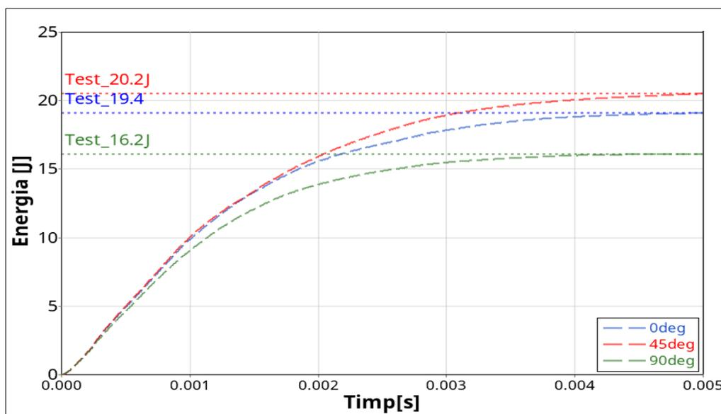
Fig. 13 Comparison of Physical Test vs. Numerical Simulation for V-Notched Specimens
