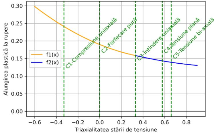
Fig. 6 Failure strain as a function of triaxiality stress state
