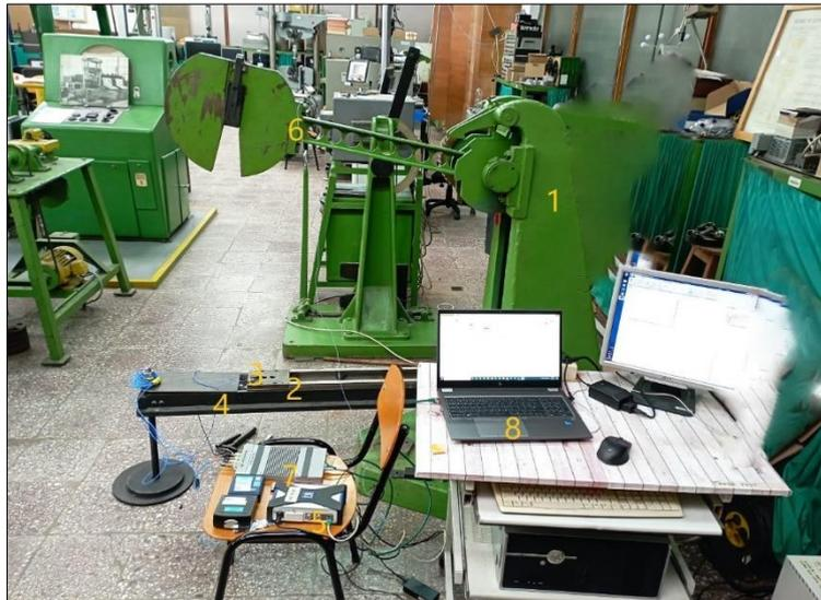
Fig. 18 Instrumented Pendulum for Dynamic Destructive Testing
