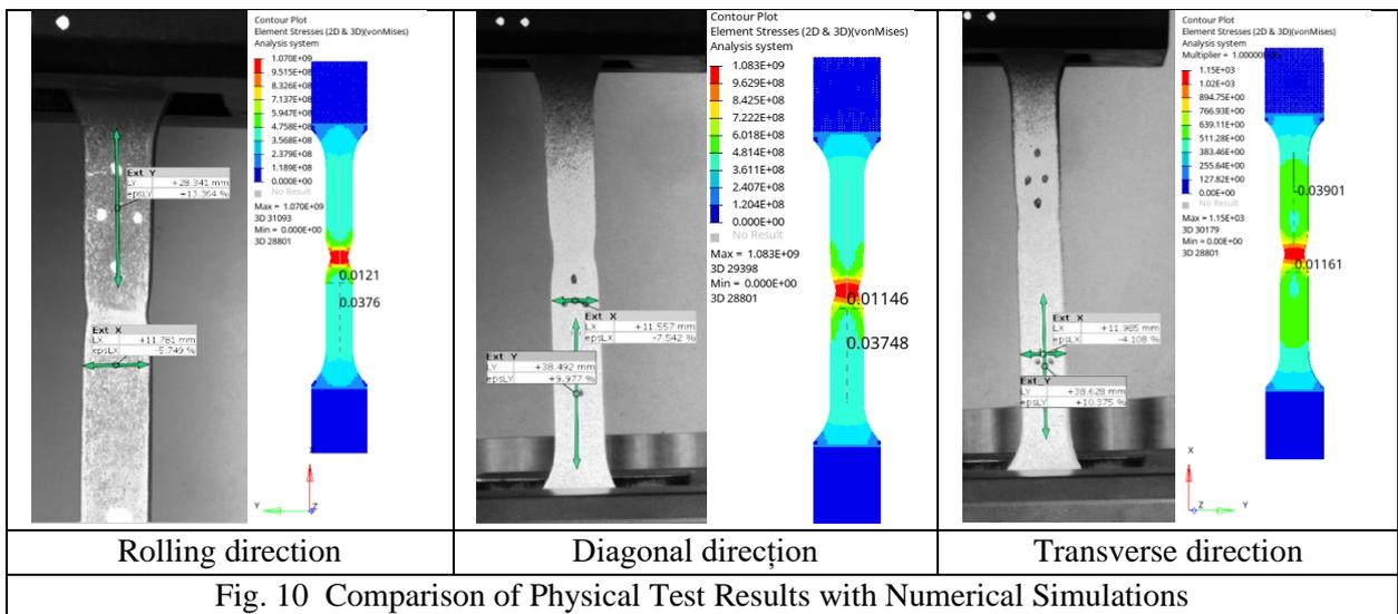
Fig. 10 Comparison of Physical Test Results with Numerical Simulations
