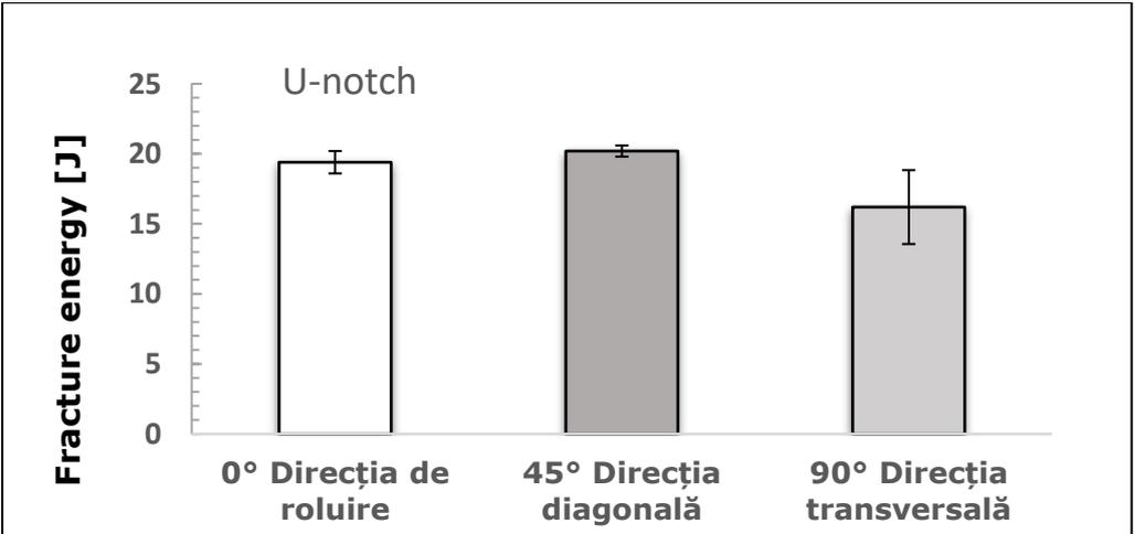
Fig. 12 Results of the Resilience Tests for U-Notched Specimens
