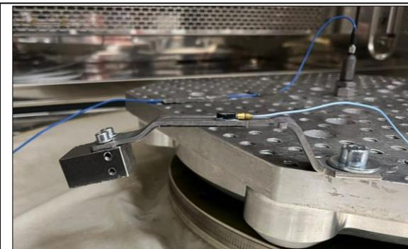
Fig. 20 High-Cycle Fatigue Testing setup
