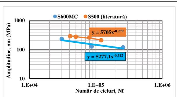
Fig. 21 The S-N curve obtained using the electrodynamic actuator for S600MC steel, compared with a fatigue curve for S500 steel [10]
