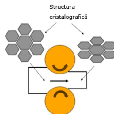
Fig. 2 Rearrangement of the Crystalline Structure Following the Rolling Process
