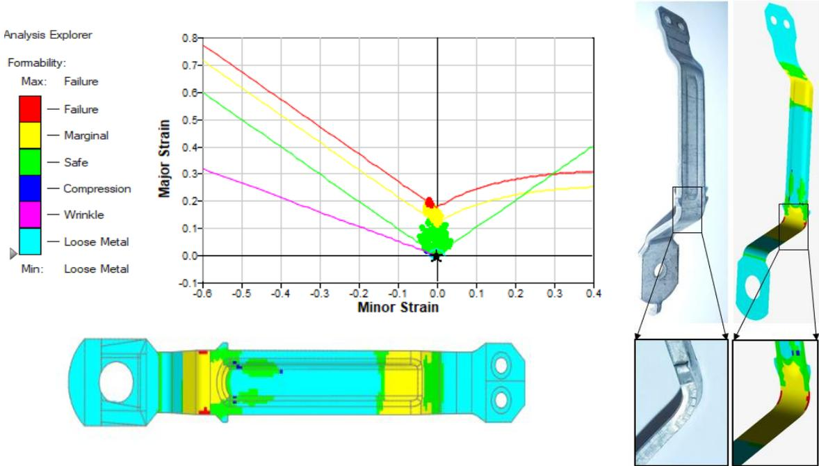
Fig. 15 Numerical Study of the Plastic Deformation Process, experimentally validated
