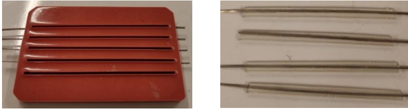
Fig. 15: Mold to apply coating and Ribbons covered with epoxy resin
