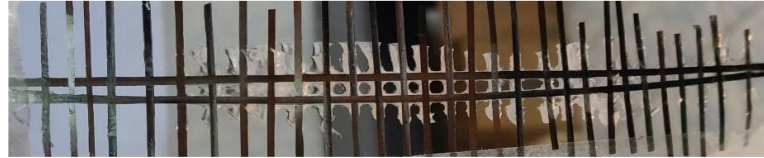
Fig. 21: Knitted ribbons used as reinforcement in the silicone matrix
