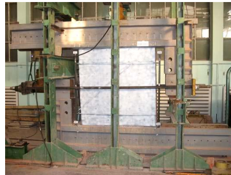
Wall retrofitted with steel shear plates
