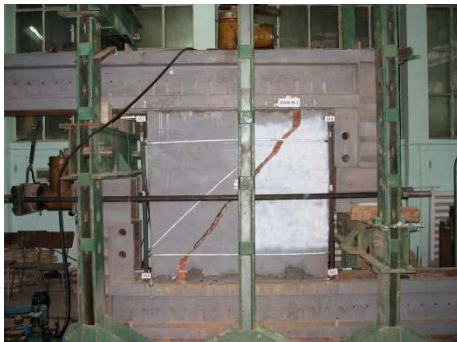
Wall retrofitted with steel wire mesh
