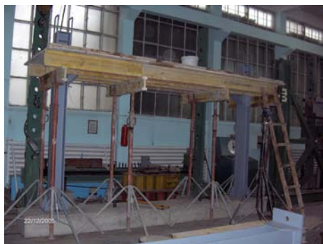
Experimental composite steel-concrete frames
