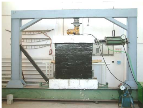
Wall retrofitted with composites
