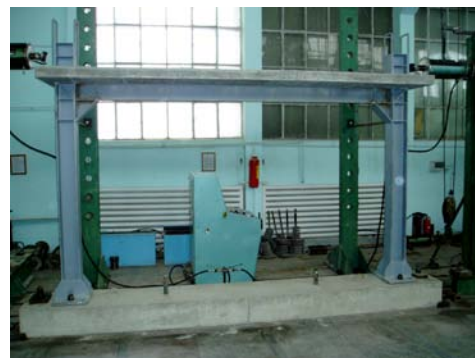
Experimental frames tested at horizontal loads
