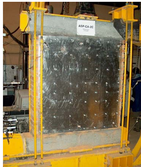
Experimental setup of a masonry panel strengthened with aluminium plates
