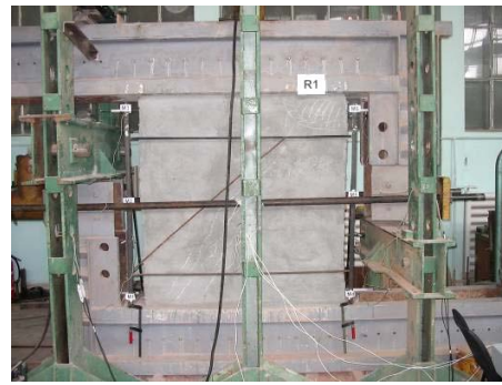
Wall retrofitted with welded wire mesh
